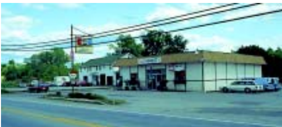
Overly wide access drives allow unpredictable turning movements, often at unsafe speeds. One narrower entrance (24 feet for two-way) will slow entering vehicles and provide space for street trees and landscaping.
