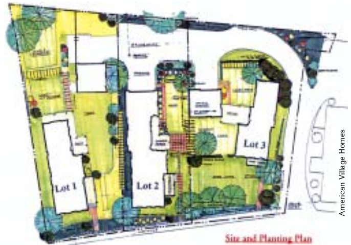
Infill project based on traditional neighborhood patterns for three single-family houses with shared driveway and rear garages on a half-acre vacant lot in the Village of Millbrook.
