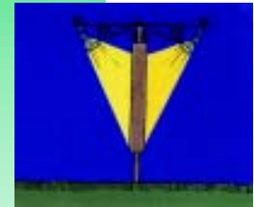
Top-mounted fixtures focus light on sign
