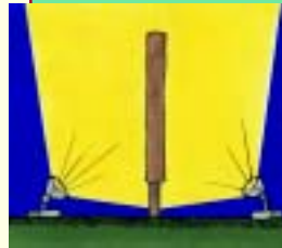
Ground floodlights uplighting sign and sky
