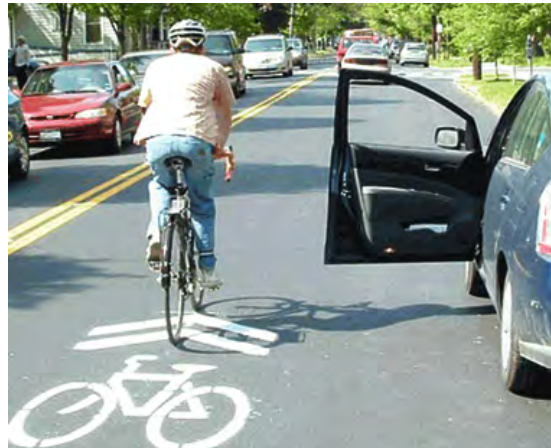
Sharrows highlight bicyclists' right to ride in the travel lane, away from hazards such as the "door zone" of parked vehicles.
