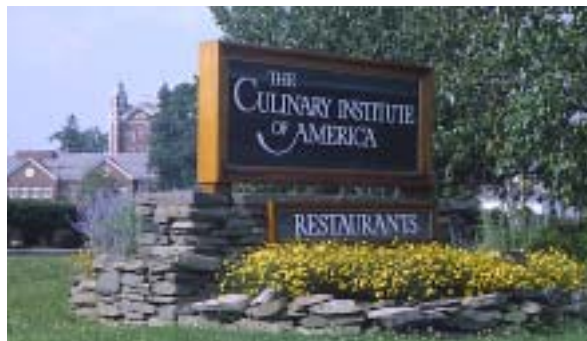
Natural looking materials are preferred, including wood and metal signs with stone, masonry, or landscaped bases.
