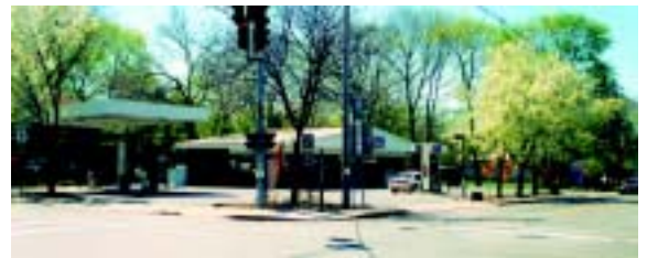
A few uses, like gas stations on small sites, may need two driveways to provide through circulation, but third or fourth curb openings, especially those too near an intersection, should be closed and the front landscaped.
