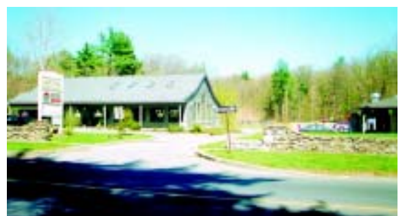
These adjacent businesses in Hyde Park share a narrow 16-foot entrance drive between buildings and a common exit onto an existing side road, along with consistent stone walls and the bulk of the parking to the rear.
