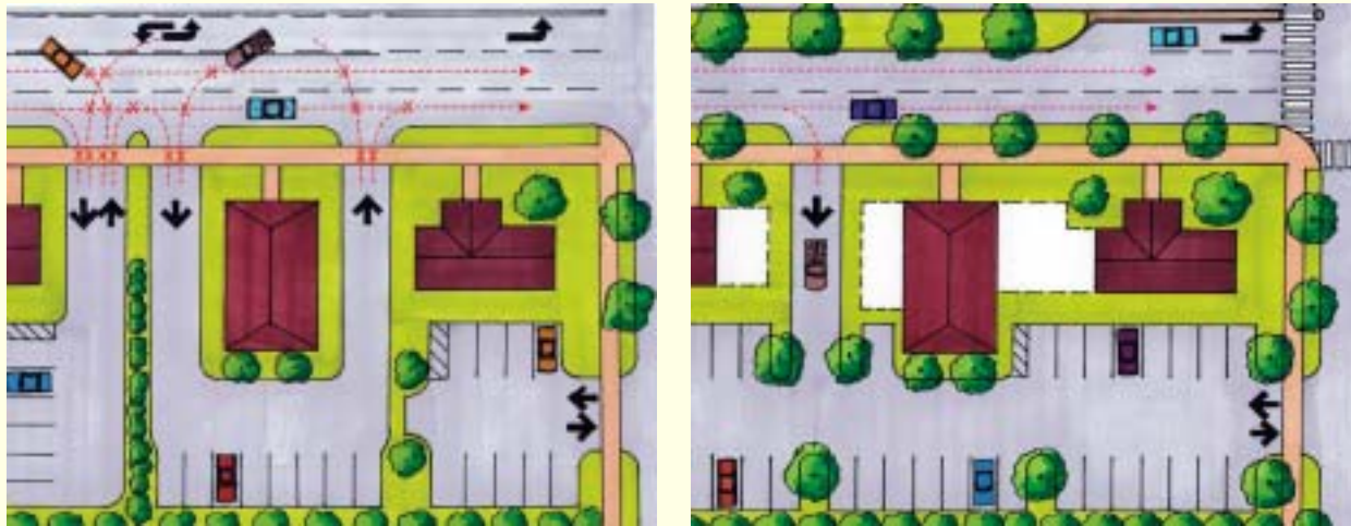
Center medians combined with shared access drives can ease congestion and dramatically reduce potential accident points (X). Fewer driveways also allow space for businesses to expand, creating a more continuous pedestrian-friendly frontage.
