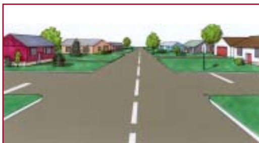
Residential streets with large setbacks and no street trees look so wide that they induce higher speeds.
